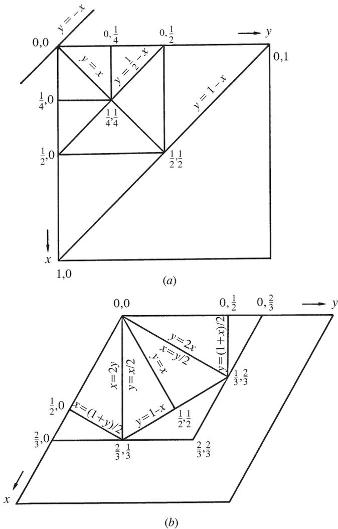
**Figure 2.1.3.11** Boundary planes of asymmetric units occurring in the space-group tables. (a) Tetragonal system. (b) Trigonal and hexagonal systems. The point coordinates refer to the vertices in the plane  $z = 0$ .
