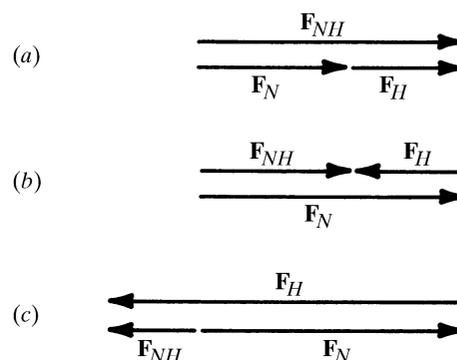
Fig. 2.3.3.1. Three different cases which can occur in the relation of the native,  $\mathbf{F}_N$ , and heavy-atom derivative,  $\mathbf{F}_{NH}$ , structure factors for centrosymmetric reflections.  $\mathbf{F}_N$  is assumed to have a phase of 0, although analogous diagrams could be drawn when  $\mathbf{F}_N$  has a phase of  $\pi$ . The crossover situation in (c) is clearly rare if the heavy-atom substitution is small compared to the native molecule, and can in general be neglected.
