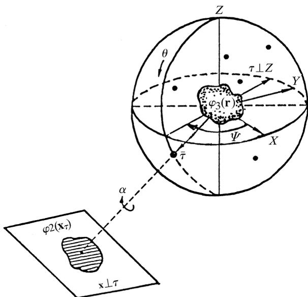
Fig. 2.5.6.2. The projection sphere and projection  $\varphi_2$  of  $\varphi_3$  along  $\tau$  onto the plane  $\mathbf{x} \perp \tau$ . The case  $\tau \perp z$  represents orthoaxial projection. Points indicate a random distribution of  $\tau$ .
