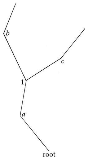
Fig. 3.3.1.2. Schematic representation of a simple branched-chain molecule with a stationary root and two extremities. The positions marked *a*, *b* and *c* are the loci of possible conformational change, here called conformons, and there is a single, numbered branch point.
