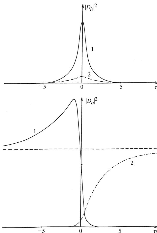
Fig. 5.1.6.2. Variation of the intensities of the reflected and refracted waves in an absorbing crystal for the 220 reflection of Si using Mo  $K\alpha$  radiation,  $t = 1$  mm ( $\mu t = 1.42$ ). Solid curve: branch 1; dashed curve: branch 2.
