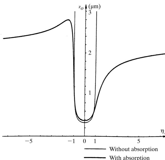
Fig. 5.1.7.3. Bragg case: thick crystals. Variation of the penetration depth with incidence angle (represented here by the dimensionless deviation parameter  $\eta$ ). Thin curve: without absorption; thick curve: with absorption for the 400 reflection of GaAs using Cu  $K\alpha$  radiation.
