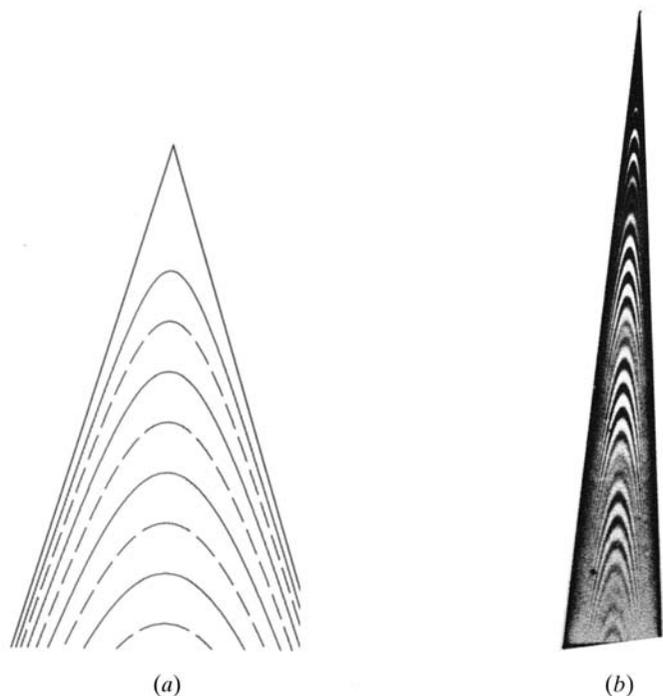
Fig. 5.1.8.5. Spherical-wave *Pendellösung* fringes observed on a wedge-shaped crystal. (a) Computer simulation (solid lines: maxima; dashed lines: minima). (b) X-ray section topograph of a wedge-shaped silicon crystal (444 reflection, Mo  $K\alpha$  radiation).
