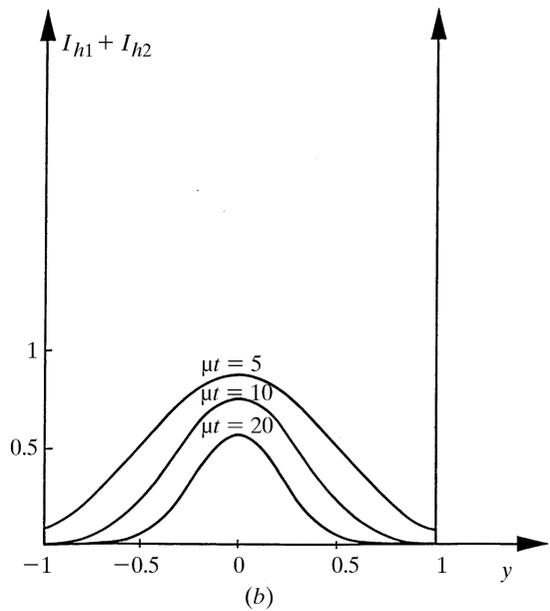
Fig. 5.1.8.3. Intensity distribution along the base of the Borrmann triangle.  $y$  is a normalized coordinate along  $BC$ . (a) Small values of  $\mu t$ . The interference (spherical-wave *Pendellösung*) between branch 1 and branch 2 is neglected. (b) Large values of  $\mu t$ .
