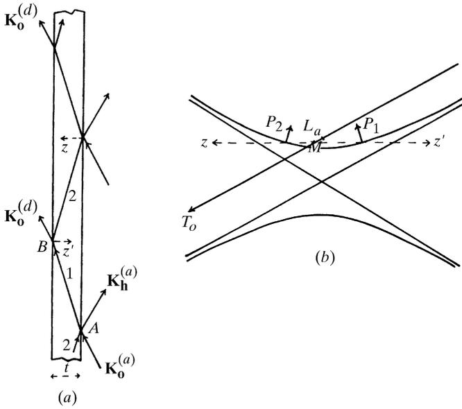
Fig. 5.1.7.4. Bragg case: thin crystals. Two wavefields propagate in the crystal. (a) Direct space; (b) reciprocal space.
