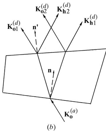
Fig. 5.1.6.3. Boundary condition for the wavevectors at the exit surface. (a) Reciprocal space. The wavevectors of the emerging waves are determined by the intersections  $M_1$ ,  $M_2$ ,  $N_1$  and  $N_2$  of the normals  $\mathbf{n}'$  to the exit surface, drawn from the tie points  $P_1$  and  $P_2$  of the wavefields, with the tangents  $T_o'$  and  $T_h'$  to the spheres centred at  $O$  and  $H$  and of radius  $k$ , respectively. (b) Direct space.
