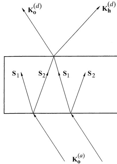
Fig. 5.1.6.4. Decomposition of a wavefield into its two components when it reaches the exit surface.  $\mathbf{S}_1$  and  $\mathbf{S}_2$  are the Poynting vectors of the two wavefields propagating in the crystal belonging to branches 1 and 2 of the dispersion surface, respectively, and interfering at the exit surface.
