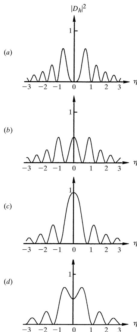
Fig. 5.1.6.6. Theoretical rocking curves in the transmission case for non-absorbing crystals and for various values of  $t/\Lambda_L$ : (a)  $t/\Lambda_L = 1.25$ ; (b)  $t/\Lambda_L = 1.5$ ; (c)  $t/\Lambda_L = 1.75$ ; (d)  $t/\Lambda_L = 2.0$ .
