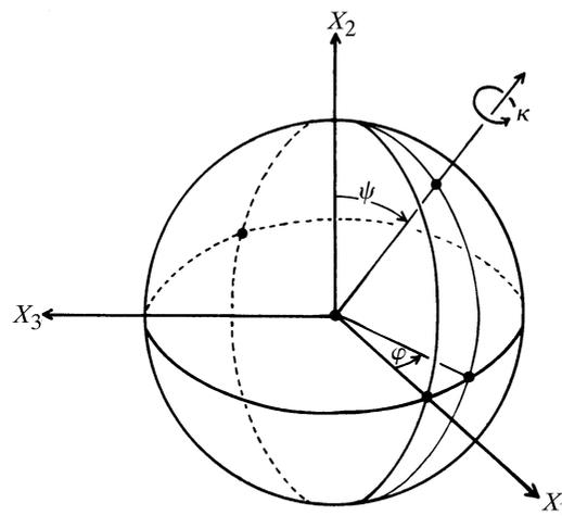
Fig. 2.3.6.4. Variables  $\psi$  and  $\phi$  are polar coordinates which specify a direction about which the axes may be rotated through an angle  $\kappa$ . [Reprinted from Rossmann & Blow (1962).]
