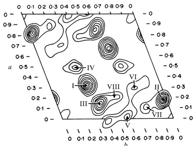
Fig. 2.3.2.2. The  $c$ -axis projection of cuprous chloride azomethane complex ( $C_2H_6Cl_2Cu_2N_2$ ). The space group is  $P1$  with one molecule per unit cell. [Adapted from and reprinted with permission from Woolfson (1970, p. 321).]
