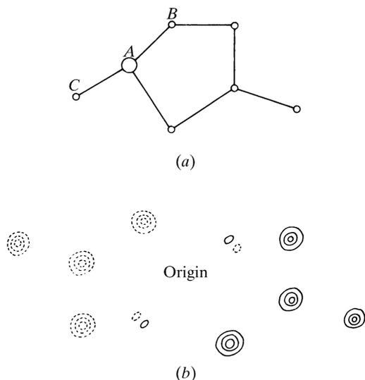
Fig. 2.3.4.1. (a) A model structure with an anomalous scatterer at A. (b) The corresponding  $P_s(\mathbf{u})$  function showing positive peaks (full lines) and negative peaks (dashed lines). [Reprinted with permission from Woolfson (1970, p. 293).]
