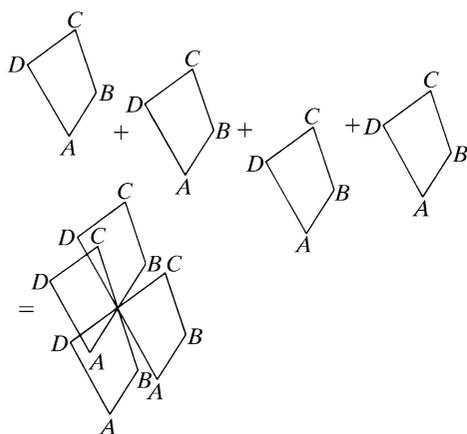
Fig. 2.3.2.3. Atoms  $ABCD$ , arranged as a quadrilateral, generate a Patterson which is the sum of the images of the quadrilateral when each atom is placed on the origin in turn.
