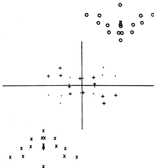
Fig. 2.3.7.2. Vectors arising from the structure in Fig. 2.3.7.1. The self-vectors of molecules  $A$  and  $B$  are represented by  $+$  and  $;$ ; the cross-vectors from molecules  $A$  to  $B$  and  $B$  to  $A$  by  $x$  and  $o$ . Triangles mark the position of  $+\Delta^{AB}$  and  $-\Delta^{AB}$ . [Reprinted from Rossmann *et al.* (1964).]
