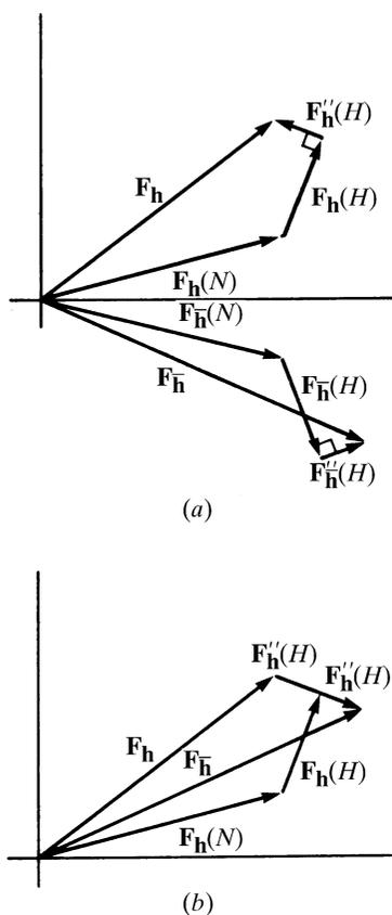
Fig. 2.3.4.2. Anomalous-dispersion effect for a molecule whose light atoms contribute  $F_h(N)$  and heavy atom  $F_h(H)$  with a small anomalous component of  $F_h''(H)$ ,  $90^\circ$  ahead of the non-anomalous  $F_h(H)$  component. In (a) is seen the construction for  $F_h$  and  $F_{\bar{h}}$ . In (b)  $F_{\bar{h}}$  has been reflected across the real axis.
