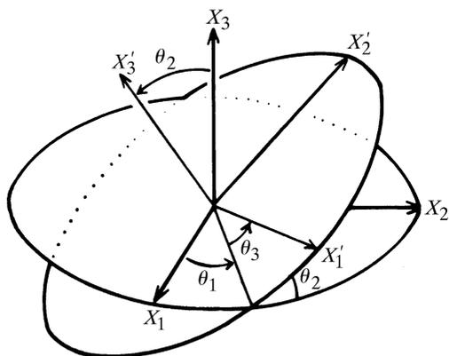
Fig. 2.3.6.3. Eulerian angles  $\theta_1, \theta_2, \theta_3$  relating the rotated axes  $X'_1, X'_2, X'_3$  to the original unrotated orthogonal axes  $X_1, X_2, X_3$ . [Reprinted from Rossmann & Blow (1962).]
