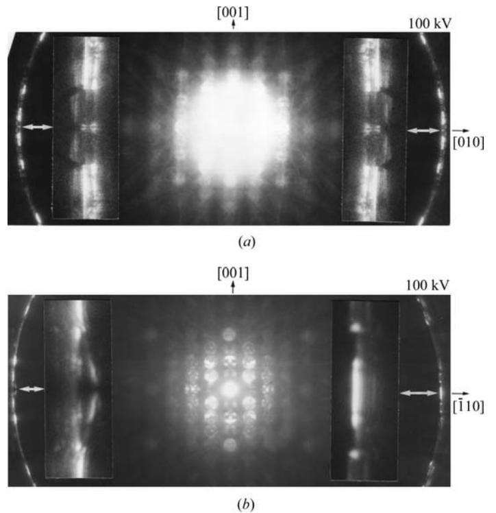
Fig. 2.5.3.14. HOLZ CBED pattern of FeS<sub>2</sub>. (a) [100] incidence: type *A* dynamical extinction lines are seen clearly in the enlarged insets. (b) [110] incidence: a type *A\** dynamical extinction line is seen clearly in the enlarged insets.
