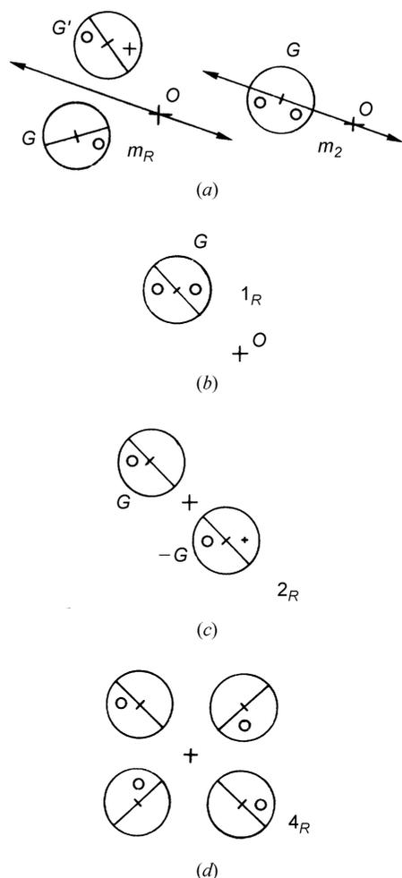
Fig. 2.5.3.2. Illustration of symmetries appearing in dark-field patterns (DPs). (a)  $m_R$  and  $m_2$ ; (b)  $1_R$ ; (c)  $2_R$ ; (d)  $4_R$ , originating from  $2'$ ,  $m'$ ,  $i$  and  $\bar{4}$ , respectively.
