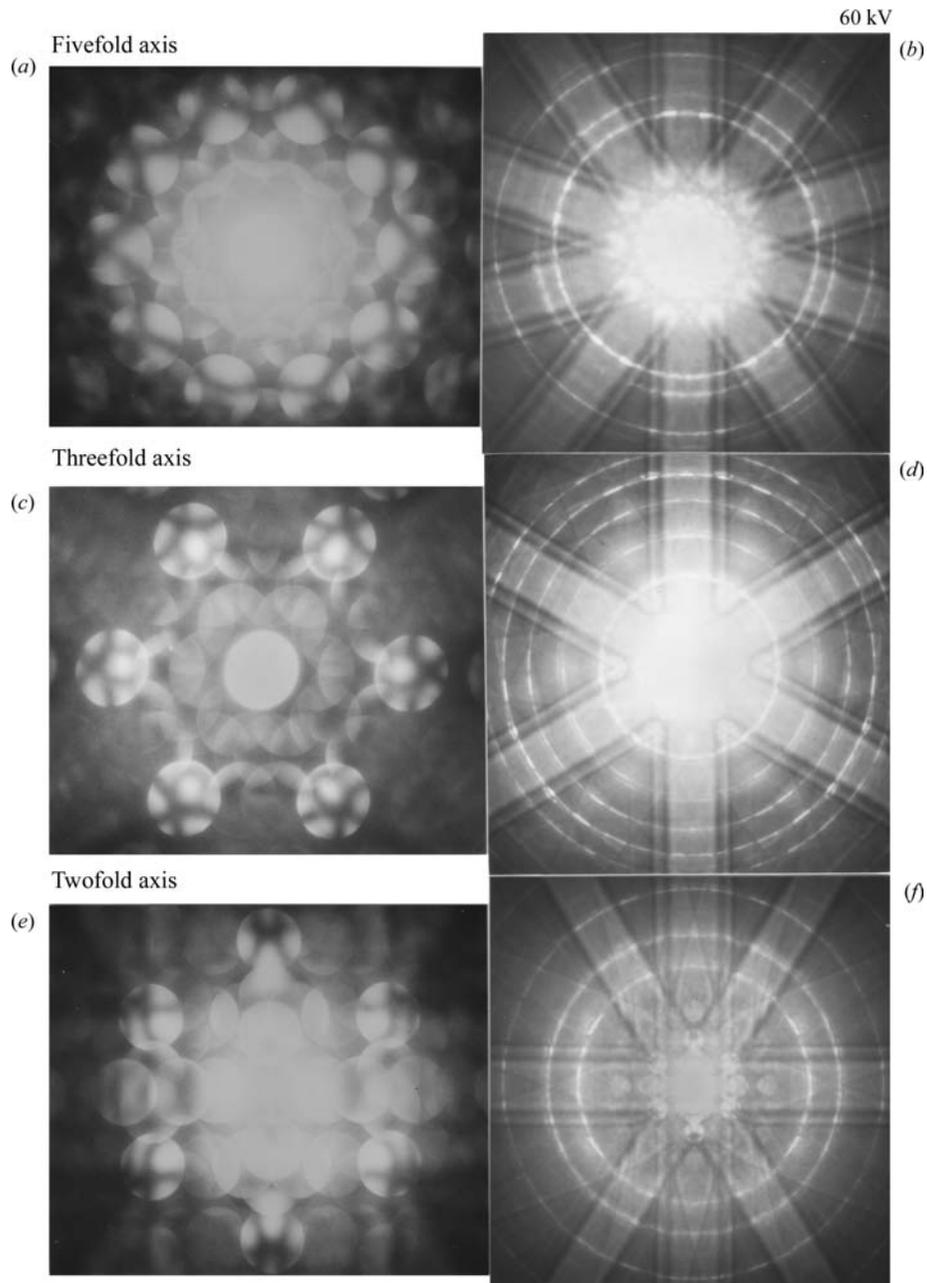
Fig. 2.5.3.24. Three pairs of ZOLZ [(a), (c) and (e)] and HOLZ [(b), (d) and (f)] CBED patterns taken at 60 kV from an area of  $\text{Al}_{74}\text{Mn}_{20}\text{Si}_6$  about 3 nm in diameter and about 10 nm thick (Tanaka, Terauchi, Suzuki *et al.*, 1987). Symmetries are (a)  $10mm$ , (b)  $5m$ , (c)  $6mm$ , (d)  $3m$ , (e)  $2mm$  and (f)  $2mm$ .
