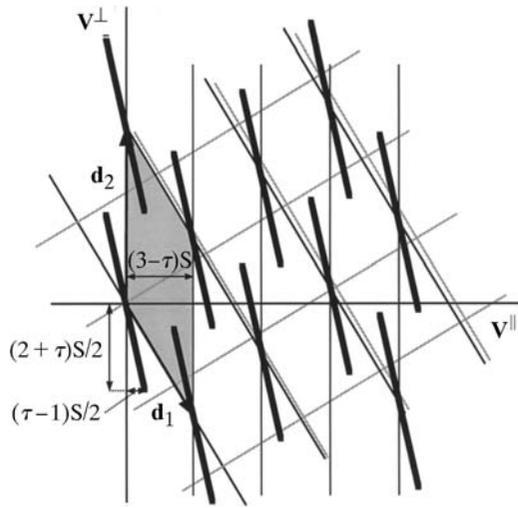
Fig. 4.6.2.11. 2D direct-space embedding of the Fibonacci chain as a modulated structure. The average period is  $(3 - \tau)S$ . The square lattice in the quasicrystal description shown in Fig. 4.6.2.8 is indicated by grey lines. The rod-like atomic surfaces are now inclined relative to  $\mathbf{V}^{\parallel}$  and arranged so as to give a saw-tooth modulation wave.
