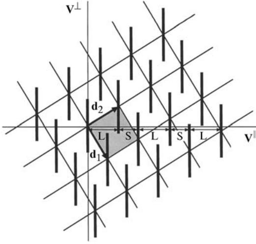
Fig. 4.6.2.8. 2D embedding of the Fibonacci chain. The short and long distances  $S$  and  $L$ , generated by the intersection of the atomic surfaces with the physical space  $\mathbf{V}^{\parallel}$ , are indicated. The atomic surfaces are represented by bars parallel to  $\mathbf{V}^{\perp}$ . Their lengths correspond to the projection of one unit cell (shaded) upon  $\mathbf{V}^{\perp}$ .
