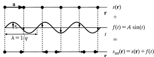
Fig. 4.6.2.1. The combination of a basic structure  $s(\mathbf{r})$ , with period  $a$ , and a sinusoidal modulation function  $f(t)$ , with amplitude  $A$ , period  $\lambda$  and  $t = \mathbf{q} \cdot \mathbf{r}$ , gives a modulated structure (MS)  $s_m(\mathbf{r})$ . The MS is aperiodic if  $a$  and  $\lambda$  are incommensurate length scales. The filled circles represent atoms.
