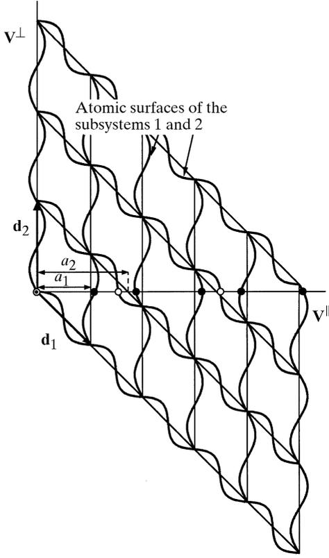
Fig. 4.6.2.5. 2D embedding of a 1D composite structure with mutual interaction of the subsystems causing modulations. Filled and empty circles represent the modulated subsystems with periods  $a_1$  and  $a_2$  of the basic subsystems, respectively. The atoms result from the parallel-space cut of the sinusoidal atomic surfaces running parallel to  $\mathbf{d}_1$  and  $\mathbf{d}_2$ .
