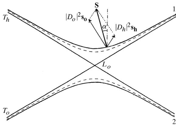
Fig. 5.1.2.5. Dispersion surface for the two states of polarization. Solid curve: polarization normal to the plane of incidence ( $C = 1$ ); broken curve: polarization parallel to the plane of incidence ( $C = \cos 2\theta$ ). The direction of propagation of the energy of the wavefields is along the Poynting vector,  $\mathbf{S}$ , normal to the dispersion surface.
