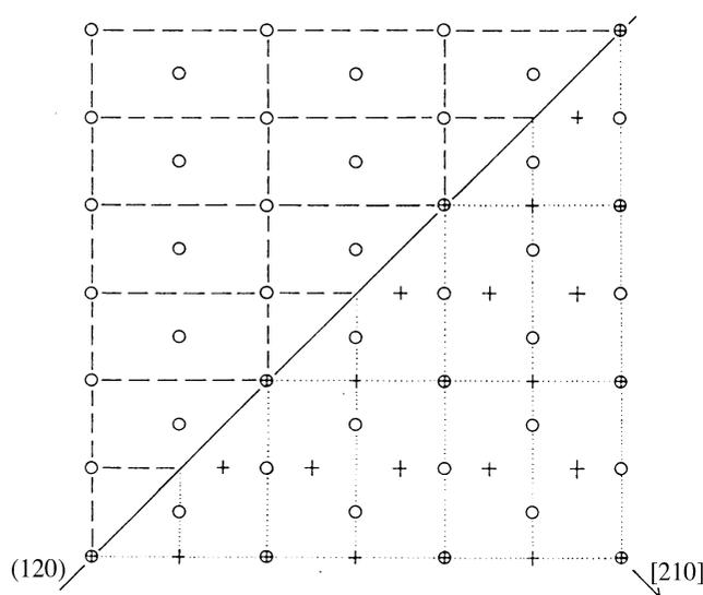
Fig. 1.3.2.3. Projection of the lattices of the twin components of an orthorhombic twinned crystal ( $oC$ ,  $b = 2a$ ) with twin index 4. The twin may be interpreted either as a rotation twin with twin axis  $[210]$  or as a reflection twin with twin plane  $(120)$ .
