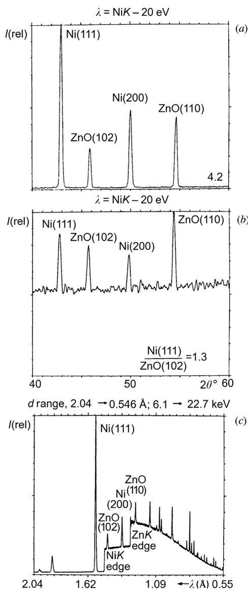
Fig. 2.3.2.3. Synchrotron-radiation patterns of a mixture of Ni and ZnO powders. Diffraction pattern using a wavelength (a) slightly longer than the Ni  $K$ -absorption edge and (b) slightly shorter. (c) High-resolution energy-dispersive diffraction (EDD) pattern.
