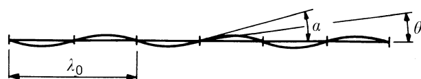
Fig. 4.2.1.8. Electron trajectory within a multipole wiggler or undulator. \lambda_0 is the spatial period, \alpha the maximum deflection angle, and \theta the observation angle. From Buras & Tazzari (1984); courtesy of ESRP.
