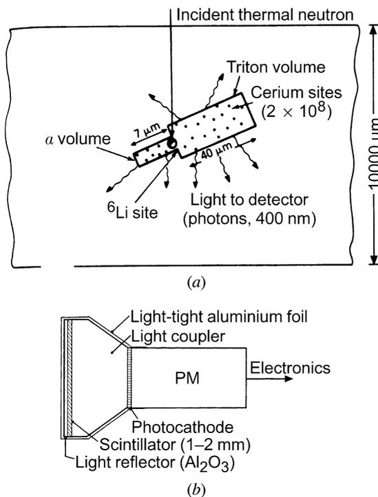
Fig. 7.3.3.3. (a) Schematic representation of the neutron capture, secondary  $\alpha$ , and triton ionization volumes, and scintillator light emission in a cerium-doped lithium silicate glass. [Reproduced from Convert & Forsyth (1983).] (b) Schematic representation of a scintillation detector.
