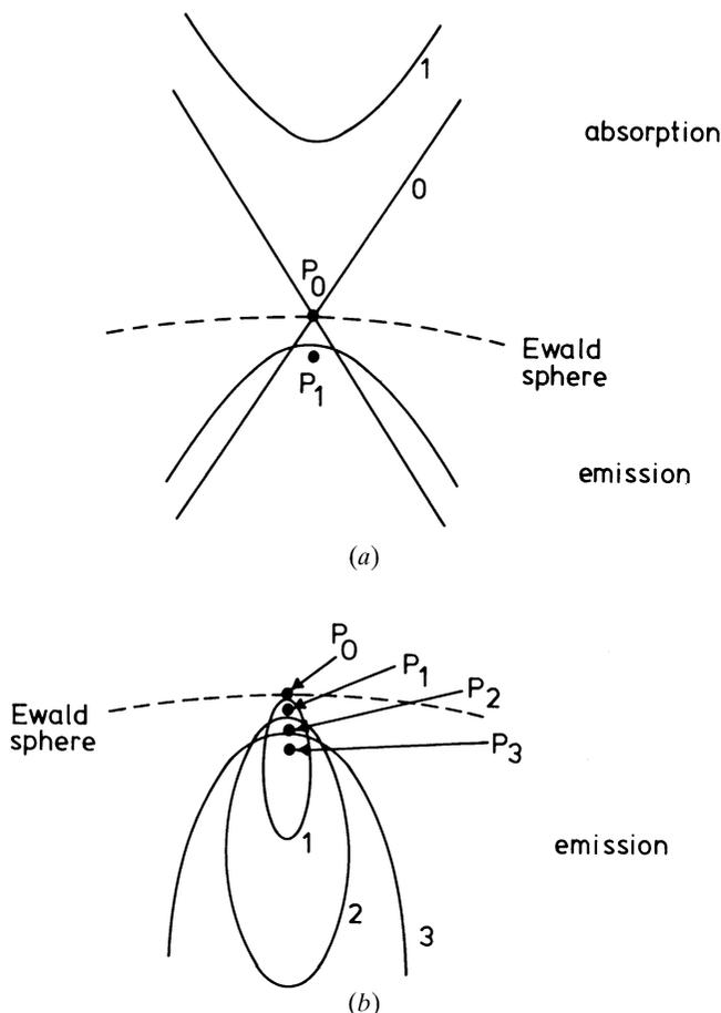
Fig. 7.4.2.3. Scattering surfaces for one-phonon scattering of neutrons: (a) for neutrons faster than sound ( $\beta < 1$ ); (b) for neutrons slower than sound ( $\beta > 1$ ). The scattering surface for X-rays is the Ewald sphere.  $P_0$ ,  $P_1$ , etc. are different positions of the reciprocal-lattice point with respect to the Ewald sphere, and the scattering surfaces are numbered to correspond with the appropriate position of  $P$ .
