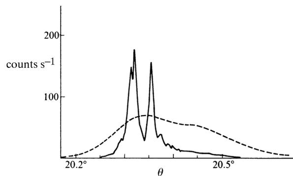
Fig. 7.4.4.2. Reflection 400 of LiH measured with a parallel beam of  $Mo K\alpha$  radiation (solid curve). The broken curve shows the reflection as convoluted by a Gaussian instrumentation function of  $2\sigma = 0.1^\circ$  and  $\theta(\alpha_2) - \theta(\alpha_1) = 0.13^\circ$ , which values are comparable with those in Fig. 7.4.4.4.
