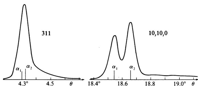
Fig. 7.4.4.4. Two reflections of beryllium acetate measured with  $MoK\alpha$ . The graphite (002) monochromator reflects in the vertical plane, while the crystal reflects in the horizontal plane. The equatorial divergence of the beam is  $0.8^\circ$ , FWHM.
