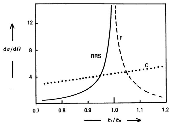
Fig. 7.4.3.3. The cross section for resonant Raman scattering (RRS) and fluorescence (F) as a function of the ratio of the incident energy,  $E$ , and the  $K$ -binding energy,  $E_B$ . The units of  $d\sigma/d\Omega$  are  $(e^2/mc^2)^2$  and the data are taken from Bannett & Freund (1975). For comparison, the intensity of Compton scattering (C) from copper through an angle of  $30^\circ$  is also shown [data taken from Hubbell *et al.* (1975)].
