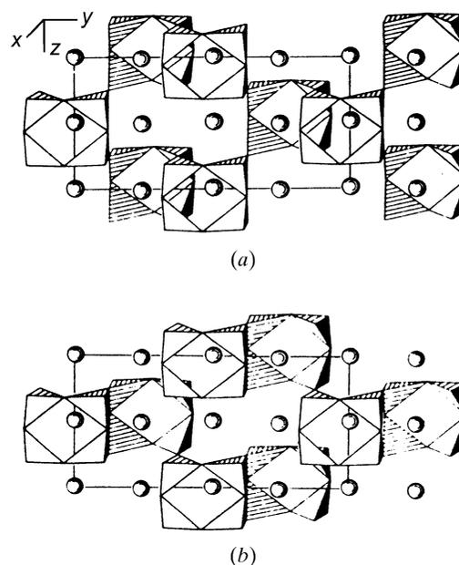
Fig. 9.2.2.20. The structural principle of  $\gamma\text{-Hg}_3\text{S}_2\text{Cl}_2$ . The shared corners of the pyramids are occupied by the Hg atoms; unshared corners are occupied by the S atoms. A pair of layers, but only the Cl atoms at their common boundary, are drawn. The two geometrically equivalent arrangements (a) and (b) are shown.
