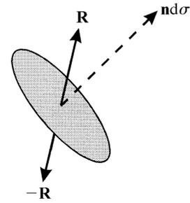
Fig. 1.3.2.1. Definition of stress: it is the limit of  $\mathbf{R} d\sigma$  when the surface element  $d\sigma$  tends towards zero.  $\mathbf{R}$  and  $\mathbf{R}'$  are the forces to which the two lips of the small surface element cut within the medium are subjected.
