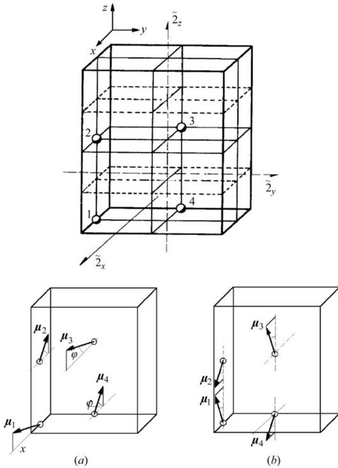
Fig. 1.5.5.4. Magnetic structures of orthoferrites and orthochromites  $RMO_3$ . (Only the transition-metal ions are shown; the setting  $Pbnm$  is used.) (a)  $G_x F_z$  weakly ferromagnetic state; (b)  $G_z F_x$  weakly ferromagnetic state.
