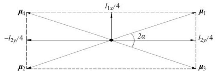
Fig. 1.5.5.6. A weakly non-collinear magnetic structure corresponding to (1.5.5.12).
