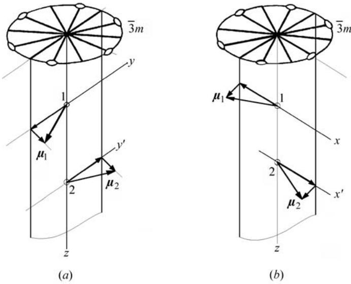
Fig. 1.5.5.1. Diagrams demonstrating two weakly ferromagnetic structures in rhombohedral crystals with two magnetic ions in the primitive cell (compare with Fig. 1.5.3.1). (a) Magnetic space group  $P2/c$ ; (b) magnetic space group  $P2'/c$ .
