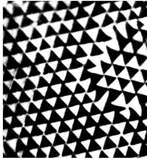
Fig. 3.4.4.5. Transmission electron microscopy (TEM) image of the incommensurate triangular ( 3 - q modulated) phase of quartz. The black and white triangles correspond to domains with domain states S_1 and S_2 , and the transition regions between black and white areas to domain walls (discommensurations). For a domain wall of a certain orientation there are no reversed domain walls with the same orientation but reversed order of black and white; the walls are, therefore, non-reversible. Domain walls in regions with regular triangular structures are related by 120 and 240° rotations about the z direction and carry parallel spontaneous polarizations (see text). Triangular structures in two regions (blocks) with different orientations of the triangles are related e.g. by 2_x and carry, therefore, antiparallel spontaneous polarizations and behave macroscopically as two ferroelectric domains with antiparallel spontaneous polarization. Courtesy of E. Snoeck, CEMES, Toulouse and P. Saint-Grégoire, Université de Toulon.
