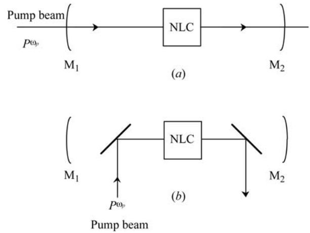
Fig. 1.7.3.18. Schematic OPO configurations.  $P^{\omega_p}$  is the pump power. (a) can be a SROPO, DROPO or TROPO and (b) can be a SROPO or DROPO, according to the reflectivity of the cavity mirrors ( $M_1, M_2$ ).
