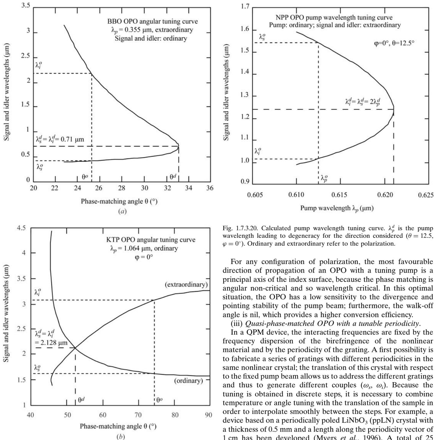
Fig. 1.7.3.19. Calculated angular tuning curves.  $\theta$  and  $\varphi$  are the spherical coordinates of the phase-matching directions.  $\theta^d$  is the phase-matching angle of the degeneracy process ( $\lambda_i^d = \lambda_s^d = 2\lambda_p$ ).  $\lambda_i^o$  and  $\lambda_s^o$  are the idler and signal wavelengths, respectively, generated at  $\theta^o$ . Ordinary and extraordinary refer to the polarization.
