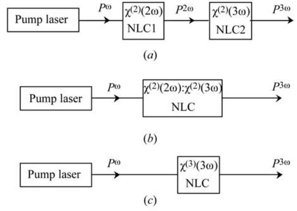
Fig. 1.7.3.16. Configurations for third harmonic generation. (a) Cascading process SHG ( $\omega + \omega = 2\omega$ ): SFG ( $\omega + 2\omega = 3\omega$ ) in two crystals NLC1 and NLC2 and (b) in a single nonlinear crystal NLC; (c) direct process THG ( $\omega + \omega + \omega = 3\omega$ ) in a single nonlinear crystal NLC.
