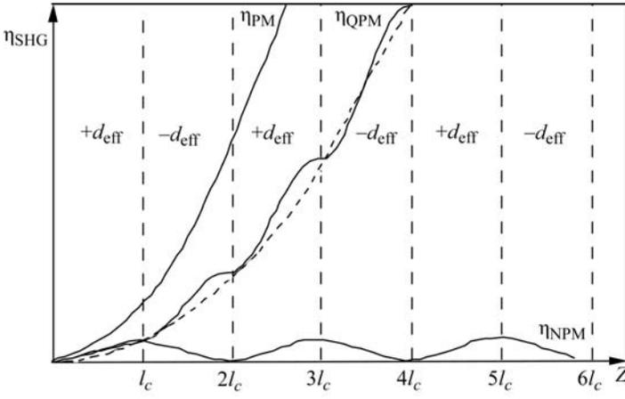
Fig. 1.7.3.7. Spatial growth evolution of second harmonic conversion efficiency,  $\eta_{\text{SHG}}$ , for non phase matching (NPM),  $\Delta k \neq 0$ , and phase matching (PM),  $\Delta k = 0$ , in a 'continuous' crystal, and for quasi phase matching (QPM) in a periodic structure. The dashed curve corresponds to  $(4/\pi^2)\eta_{\text{PM}}(Z)$  where  $\eta_{\text{PM}}$  is the conversion efficiency of the phase-matched SHG.  $l_c = \pi/\Delta k$  is the coherence length.
