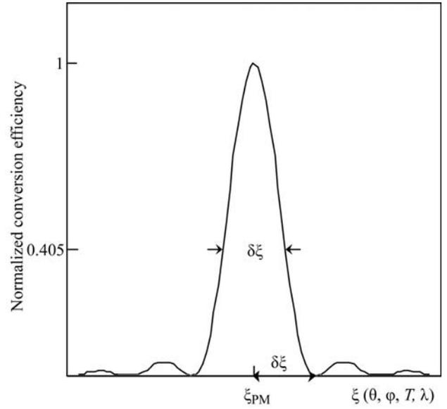
Fig. 1.7.3.8. Conversion efficiency evolution as a function of  $\xi$  for a given crystal length.  $\xi$  denotes the angle ( $\theta$  or  $\varphi$ ), the temperature ( $T$ ) or the wavelength ( $\lambda$ ).  $\xi_{\text{PM}}$  represents the parameter allowing phase matching.
