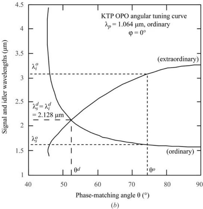
Fig. 1.7.3.19. Calculated angular tuning curves.  $\theta$  and  $\varphi$  are the spherical coordinates of the phase-matching directions.  $\theta^d$  is the phase-matching angle of the degeneracy process ( $\lambda_i^d = \lambda_s^d = 2\lambda_p$ ).  $\lambda_i^o$  and  $\lambda_s^o$  are the idler and signal wavelengths, respectively, generated at  $\theta^o$ . Ordinary and extraordinary refer to the polarization.
