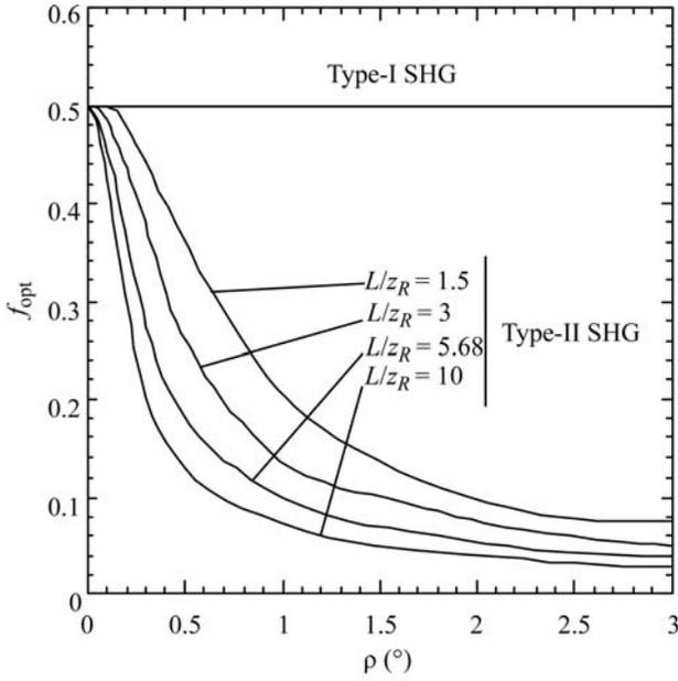
Fig. 1.7.3.12. Position  $f_{\text{opt}}$  of the beam waist for different values of walk-off angles and  $L/z_R$ , leading to an optimum SHG conversion efficiency. The value  $f_{\text{opt}} = 0.5$  corresponds to the middle of the crystal and  $f_{\text{opt}} = 0$  corresponds to the entrance surface (Fève & Zondy, 1996).
