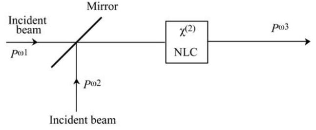
Fig. 1.7.3.17. Frequency up-conversion process  $\omega_1 + \omega_2 = \omega_3$ . The beam at  $\omega_1$  is mixed with the beam at  $\omega_2$  in the nonlinear crystal NLC in order to generate a beam at  $\omega_3$ .  $P^{\omega_1, \omega_2, \omega_3}$  are the different powers.
