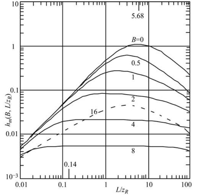
Fig. 1.7.3.13. Optimum walk-off function  $h_m(B, L)$  as a function of  $L/z_R$  for various values of  $B = (1/2)\rho\{(k_o^\omega + k_e^\omega)/2\}L^{1/2}$ . The curve at  $B = 0$  is the same for both type-I and type-II phase matching. The full lines at  $B \neq 0$  are for type II and the dashed line at  $B = 16$  is for type I. (From Zondy, 1990).
