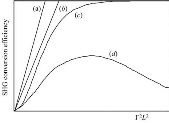
Fig. 1.7.3.15. Schematic SHG conversion efficiency for different situations of pump depletion and dephasing. (a) No depletion, no dephasing,  $\eta = \Gamma^2 L^2$ ; (b) no depletion with constant dephasing  $\delta$ ,  $\eta = \Gamma^2 L^2 \sin^2 c^2 \delta$ ; (c) depletion without dephasing,  $\eta = \tanh^2(\Gamma L)$ ; (d) depletion and dephasing,  $\eta = \eta_m \text{sn}^2(\Gamma L/v_b, v_b^4)$ .
