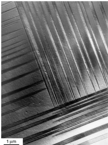
Fig. 3.4.1.4. Transmission electron microscopy image of the ferroelastic domain structure in a \text{YBa}_2\text{Cu}_3\text{O}_{7-y} crystal (Rosová, 1999). Courtesy of A. Rosová, Institute of Electrical Engineering, SAS, Bratislava. There are two systems ('complexes'), each of which is formed by almost parallel ferroelastic domain walls with needle-like tips. The domain walls in one complex are nearly perpendicular to the domain walls in the other complex.
