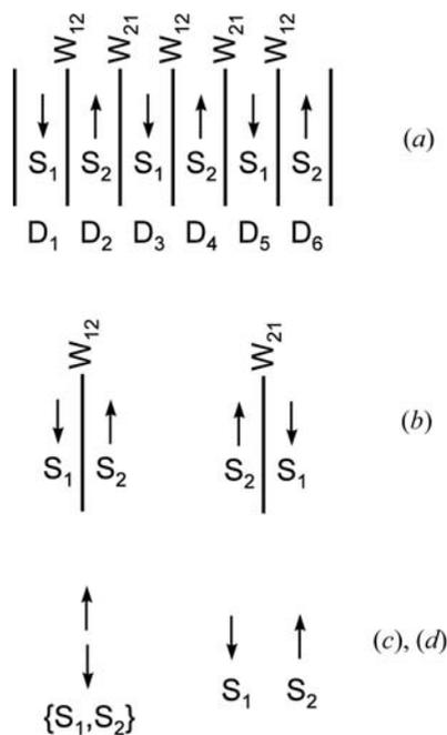
Fig. 3.4.2.1. Hierarchy in domain-structure analysis. (a) Domain structure consisting of domains  $D_1, D_2, \dots, D_6$  and domain walls  $W_{12}$  and  $W_{21}$ ; (b) domain twin and reversed twin (with reversed order of domain states); (c) domain pair consisting of two domain states  $S_1$  and  $S_2$ ; (d) domain states  $S_1$  and  $S_2$ .
