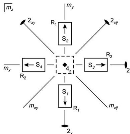
Fig. 3.4.2.2. Exploded view of single-domain states  $S_1, S_2, S_3$  and  $S_4$  (solid rectangles with arrows of spontaneous polarization) formed at a phase transition from a parent phase with symmetry  $G = 4_z/m_z m_x m_{xy}$  to a ferroic phase with symmetry  $F_1 = 2_x m_y m_z$ . The parent phase is represented by a dashed square in the centre with the symmetry elements of the parent group  $G = 4_z/m_z m_x m_{xy}$  shown.
