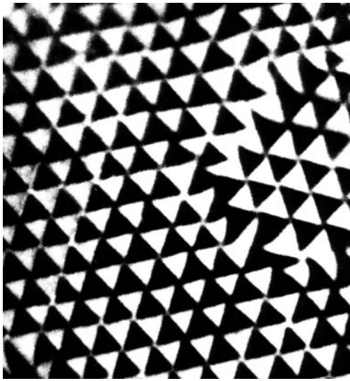
Fig. 3.4.4.5. Transmission electron microscopy (TEM) image of the incommensurate triangular ( 3 - q modulated) phase of quartz. The black and white triangles correspond to domains with domain states \mathbf{S}_1 and \mathbf{S}_2 , and the transition regions between black and white areas to domain walls (discommensurations). For a domain wall of a certain orientation there are no reversed domain walls with the same orientation but reversed order of black and white; the walls are, therefore, non-reversible. Domain walls in regions with regular triangular structures are related by 120^\circ and 240^\circ rotations about the z direction and carry parallel spontaneous polarizations (see text). Triangular structures in two regions (blocks) with different orientations of the triangles are related e.g. by 2_x and carry, therefore, antiparallel spontaneous polarizations and behave macroscopically as two ferroelectric domains with antiparallel spontaneous polarization. Courtesy of E. Snoeck, CEMES, Toulouse and P. Saint-Grégoire, Université de Toulon.
