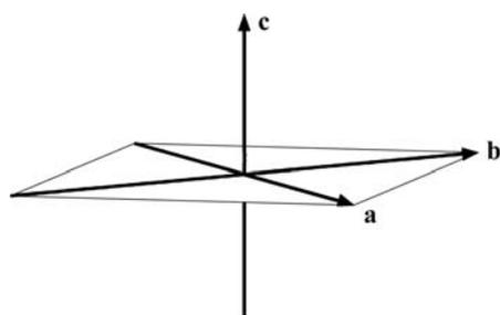
Fig. 1.2.1.2. Monoclinic/orthogonal basis vectors. For the monoclinic/orthogonal subdivision,  $\alpha = \beta = 90^\circ$  and the plane containing the **a** and **b** non-lattice basis vectors is *orthogonal* to the lattice basis vector **c**.
