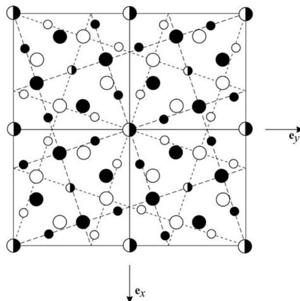
Fig. 5.2.5.3. A classical example of a bicrystal (Vlachavas, 1985).
