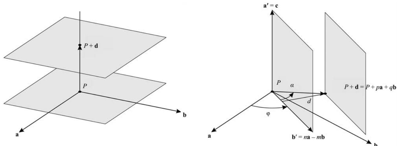
Fig. 5.2.2.2. Monoclinic/orthogonal (left) and monoclinic/inclined (right) scanning.
