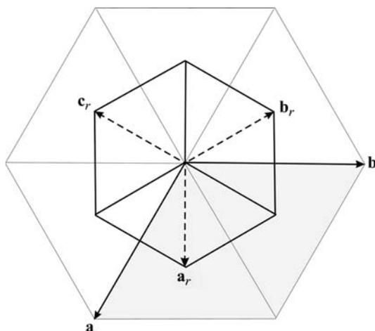
Fig. 5.2.4.4. The relationship between hexagonal and rhombohedral bases in the obverse setting.
