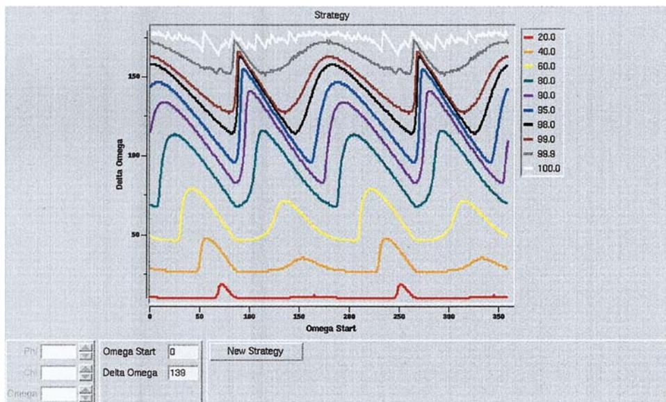
Fig. 11.4.10.1. The strategy program as implemented in the *HKL* package. The colours of the lines reflect different data-completeness goals. The y axis is the total oscillation range necessary to achieve a particular completeness goal. The x axis shows the starting position of the spindle axis.
