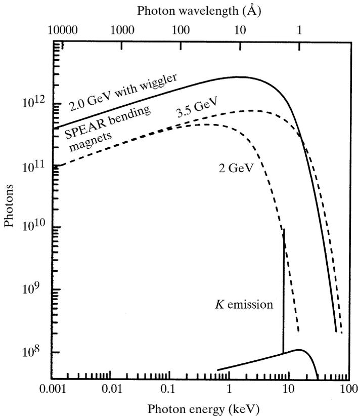
Fig. 6.1.2.3. Comparison of the spectra from the storage ring SPEAR in photons  $\text{s}^{-1} \text{mA}^{-1} \text{mrad}^{-1}$  per 1% band pass (1978 performance) and a rotating-anode X-ray generator, showing the Cu *K* emission line and the *Bremsstrahlung*. Reproduced with permission from Nagel (1980). Copyright (1980) New York Academy of Sciences.
