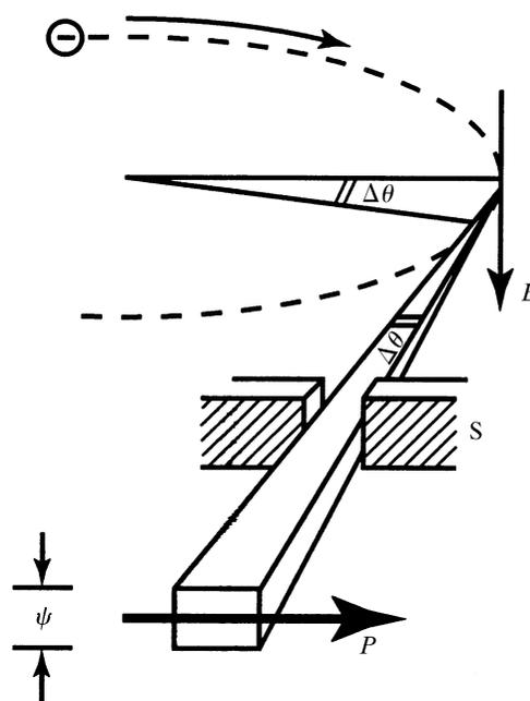
Fig. 6.1.2.2. Synchrotron radiation emitted by a relativistic electron travelling in a curved trajectory.  $B$  is the magnetic field perpendicular to the plane of the electron orbit;  $\psi$  is the natural opening angle in the vertical plane;  $P$  is the direction of polarization. The slit,  $S$ , defines the length of the arc of angle,  $\Delta\theta$ , from which the radiation is taken. From Buras & Tazzari (1984).
