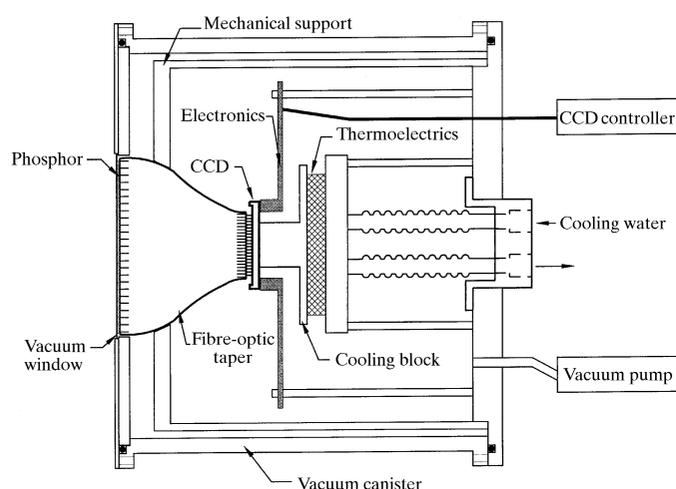
Fig. 7.2.1.1. Schematic of a single-module CCD detector. The thin phosphor screen is behind a light- and vacuum-tight vacuum window and is coupled to a fibre-optic taper, which is, in turn, coupled to a CCD. The CCD is thermoelectrically cooled to 213 K and housed in a vacuum cryostat. Reproduced with permission from Tate *et al.* (1995). Copyright (1995) International Union of Crystallography.
