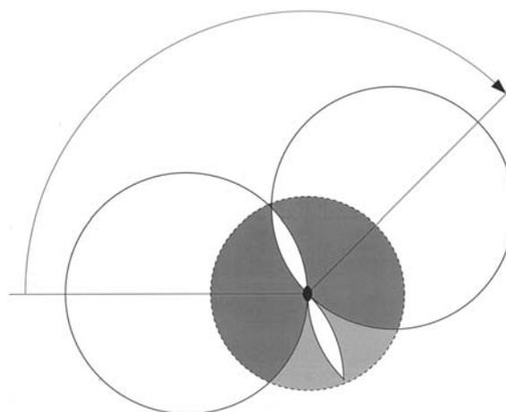
Fig. 9.1.7.2. Rotation of a triclinic crystal by  $135^\circ$  is not sufficient to obtain totally complete data. At high resolution the completeness is higher than at low resolution, where a full  $180^\circ$  rotation is required.
