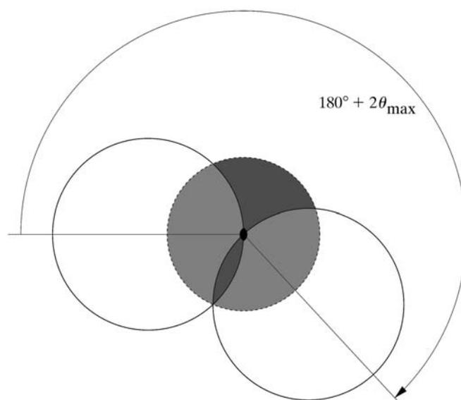
Fig. 9.1.7.6. For data containing an anomalous signal, when both Bijvoet mates have to be measured,  $180^\circ$  rotation of a triclinic crystal is not sufficient and at least an additional  $2\theta_{\max}$  is required.
