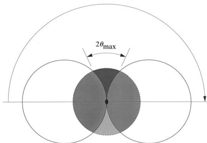
Fig. 9.1.7.1. Rotation of a triclinic crystal by  $180^\circ$  in the X-ray beam, represented as rotating the Ewald sphere with a stationary crystal, projected along the rotation axis. For the purpose of analysing the relation of data completeness to crystal symmetry and orientation both representations are equivalent.
