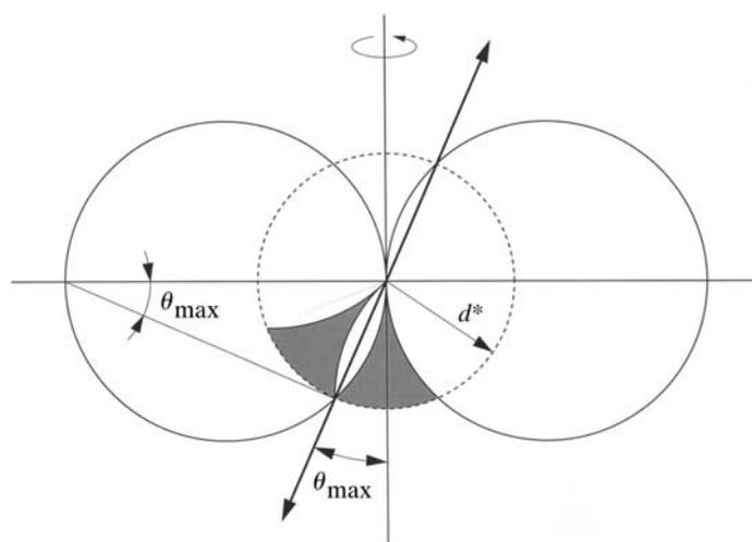
Fig. 9.1.7.10. If the crystal has a symmetry axis, it should be skewed from the rotation axis by at least  $\theta_{\text{max}}$  to be able to collect the reflections equivalent to those in the blind region.
