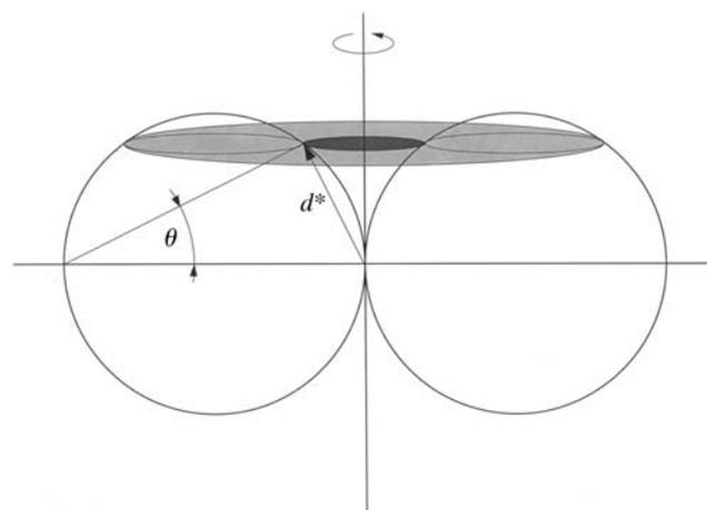
Fig. 9.1.7.7. Rotation by  $360^\circ$  leaves the part of the reciprocal space in the blind region unmeasured, since the reflections near the rotation axis do not cross the surface of the Ewald sphere. The rotation axis in this projection lies vertically in the plane of the figure.
