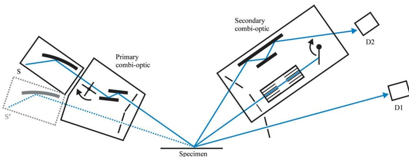
**Figure 2.1.24** Example of the use of highly sophisticated incident- and diffracted-beam combi-optics in combination with a rotatable X-ray source and a double detector arm. This setup enables two different incident-beam and four different diffracted-beam paths, and thus provides a choice between eight different beam paths, depending on the properties of the specimen and the requirements of the application. S: X-ray source, S': X-ray source rotated by about  $5^\circ$ , D1, D2: detectors.
