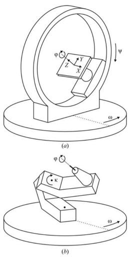
**Figure 2.1.9** Geometric definition of the Eulerian and kappa geometries with identical specimen orientation in space. (a) Specimen rotation and translation in a Eulerian cradle equipped with an XYZ stage, (b) specimen rotation on a kappa stage.
