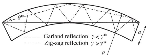
**Figure 2.3.13** Plan of a curved neutron guide, indicating different possible neutron paths, labelled ‘garland’ and ‘zig-zag’. Only the longer-wavelength neutrons can travel the zig-zag path because the glancing angles on this path (which must be less than the critical angle) are greater. In this schematic, the glancing angles, the width and the curvature have all been exaggerated. [From Section 4.4.2 of Volume C (Anderson & Schärpf, 2006).]
