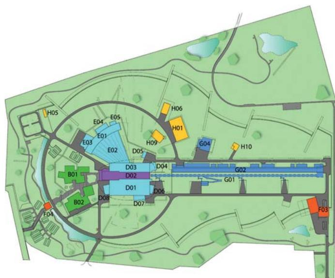
**Figure 2.3.12** Schematic diagram of the ESS facility. The proton beam enters at the right, strikes the target and liberates neutrons for instruments in the three neutron experiment halls. (Image courtesy of the ESS.)
