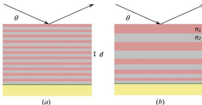
**Figure 2.3.14** Schematic diagrams of (a) a multilayer monochromator and (b) a neutron supermirror.
