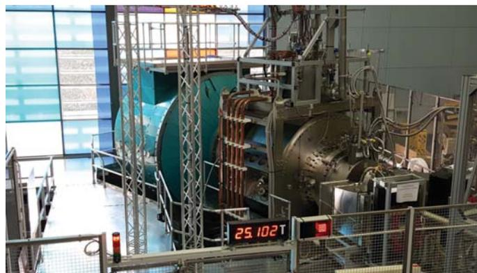
**Figure 2.8.13** The High Magnetic Field Facility for Neutron Scattering at the Helmholtz-Zentrum Berlin has two main components: the High Field Magnet (HFM) and the Extreme Environment Diffractometer (EXED). Courtesy of Dr O. Prokhnenko.
