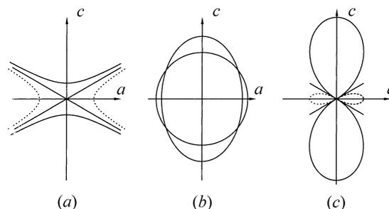
Fig. 1.4.1.1. Sections ( $ac$  plane) of representation surfaces for a trigonal (or tetragonal or hexagonal) crystal with  $\alpha_{11} = \alpha_{22} = -1$  and  $\alpha_{33} = +3 \times 10^{-5} \text{ K}^{-1}$  (similar to calcite). (a) Quadric, (b) strain ellipsoid (greatly exaggerated), (c) polar diagram. The  $c$  axis is the axis of revolution. Sectors with negative expansions are dashed.
