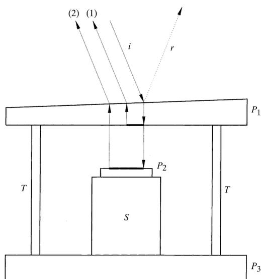
Fig. 1.4.3.1. Schematic diagram of a Fizeau interferometer.
