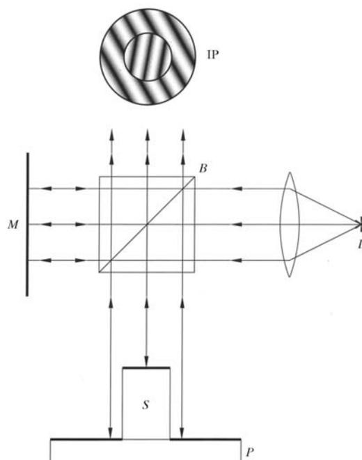
Fig. 1.4.3.2. Schematic diagram of a Michelson interferometer.
